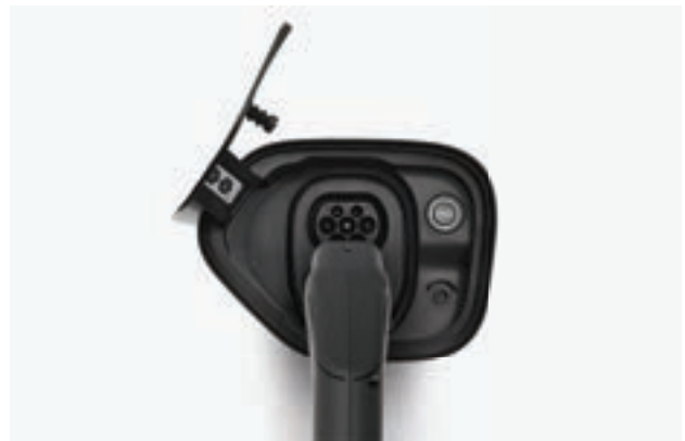
Insert the charging plug into the car's charging port (maximum 4 meters from the One).
