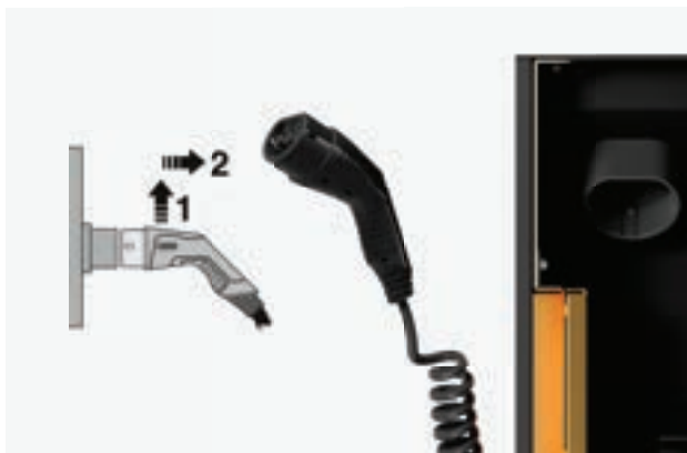
Remove the charging cable from the holder (Wall Plus - Plug).
