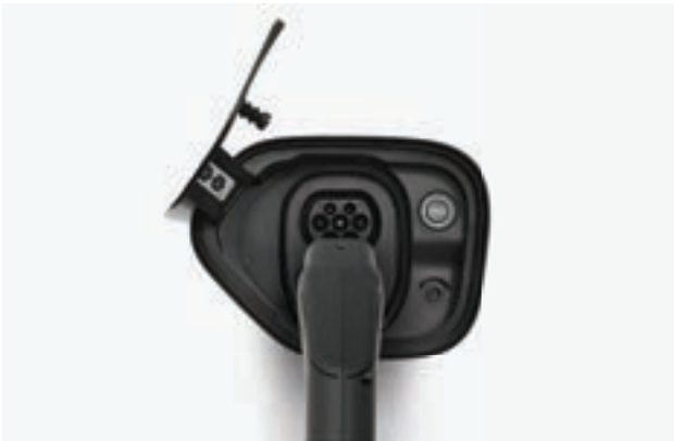
Insert the charging plug into the car’s charging port.
