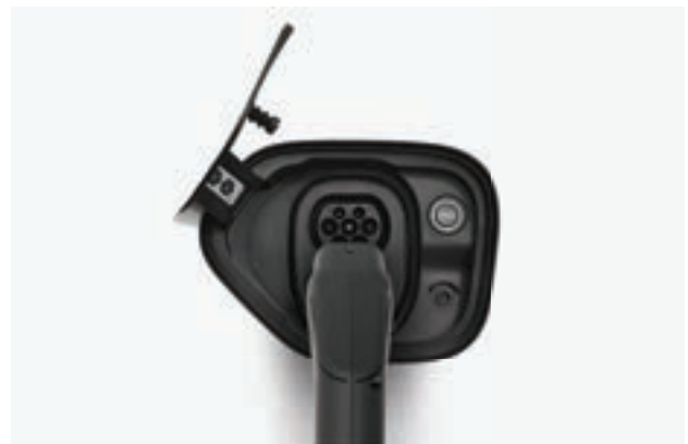
Insert the charging plug into the car's charging port.
